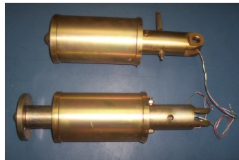
Fig 3.1: PSOM Separation Mechanism
