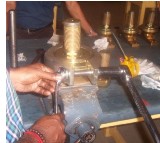
Fig 3.2: Ball-socket Joint Lapping
