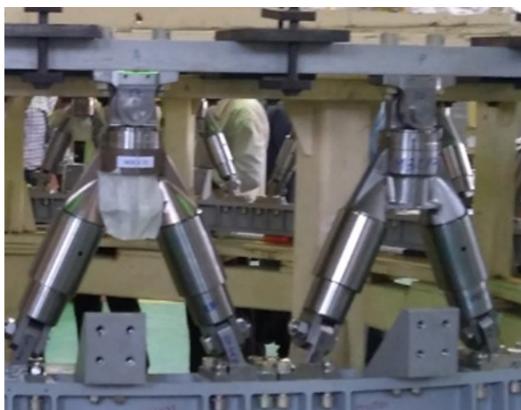
Fig. 3.24 Assembly of active & passive units of L110 Separation system
