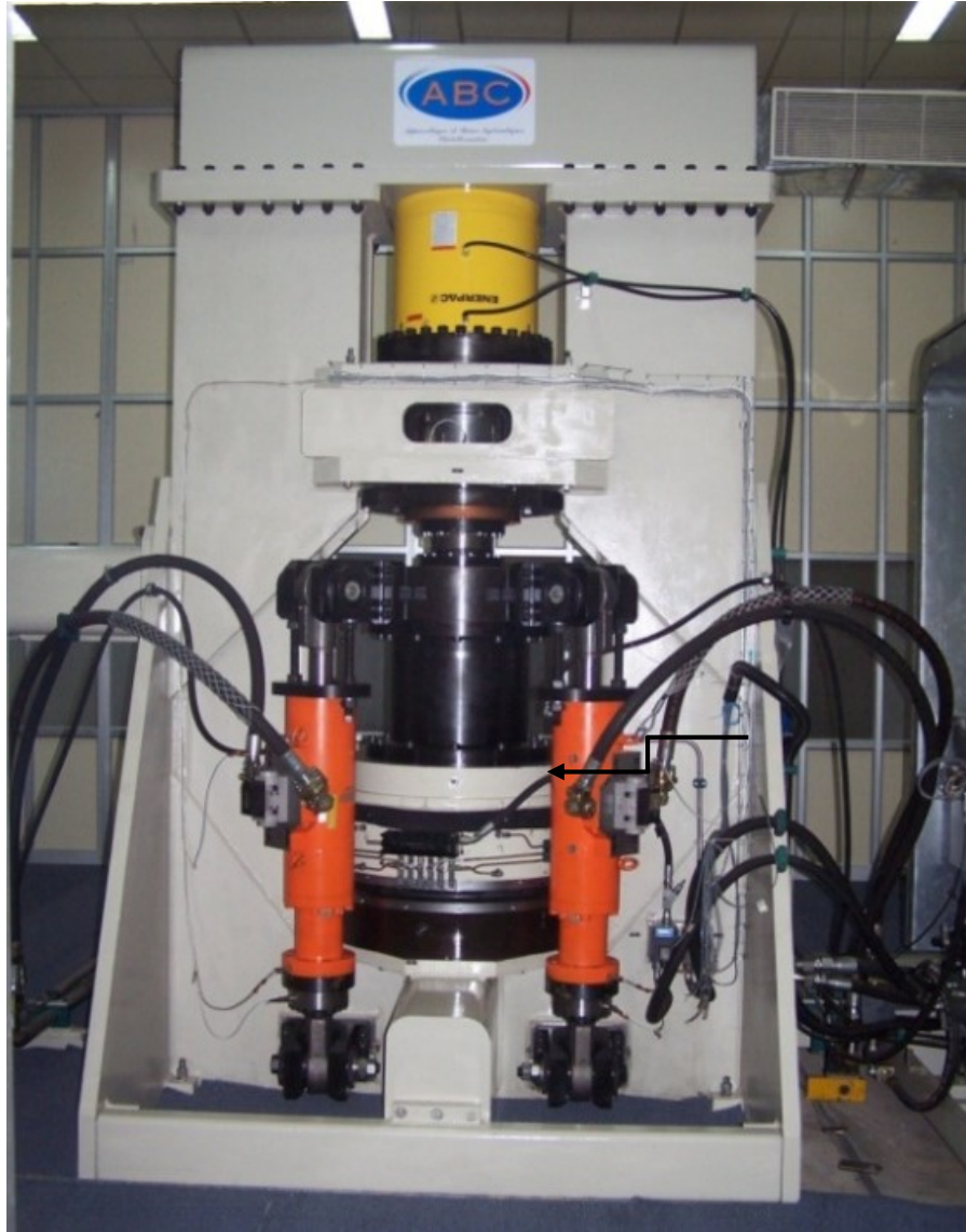
Fig. 3.23 Bearing test rig setup
