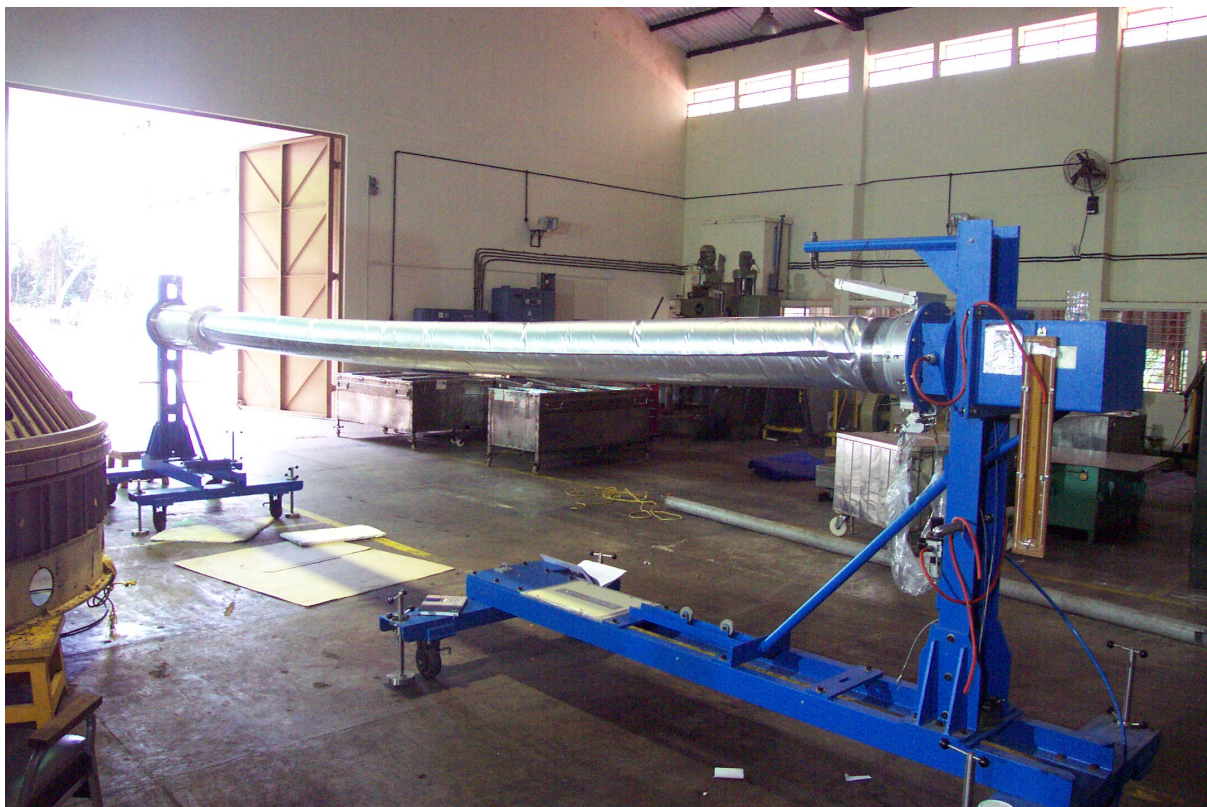
Figure 3.26: PCU COOLING HOSE PRESSURE TEST
