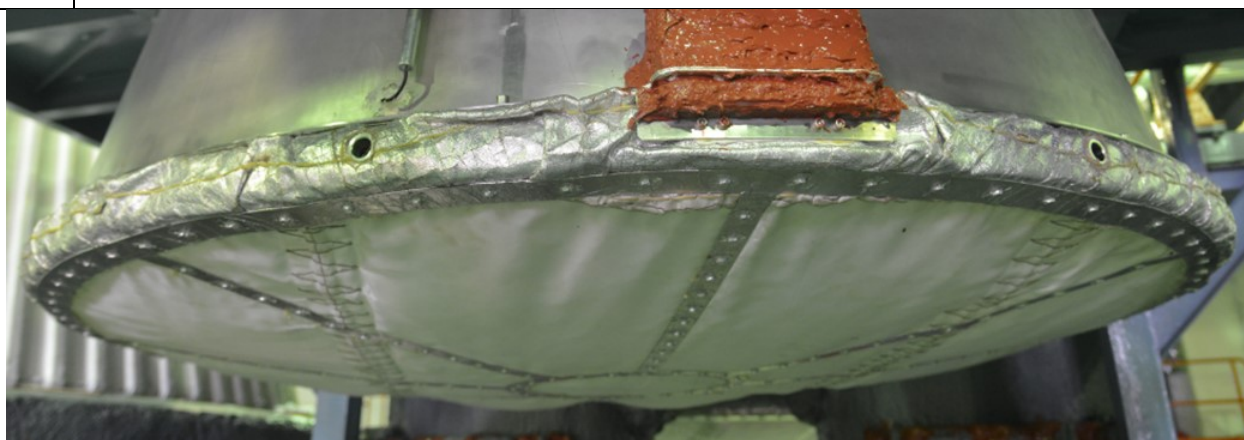
Fig.3.25 Nozzle closure system assembly with L110 Nozzle
