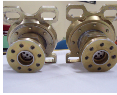
Fig 3.6: Ball lock assembly
