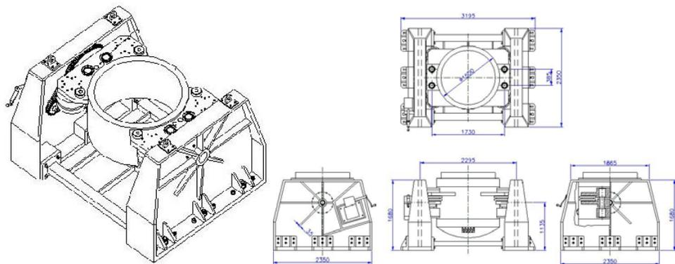
Figure 4. Shaker Suspension System
